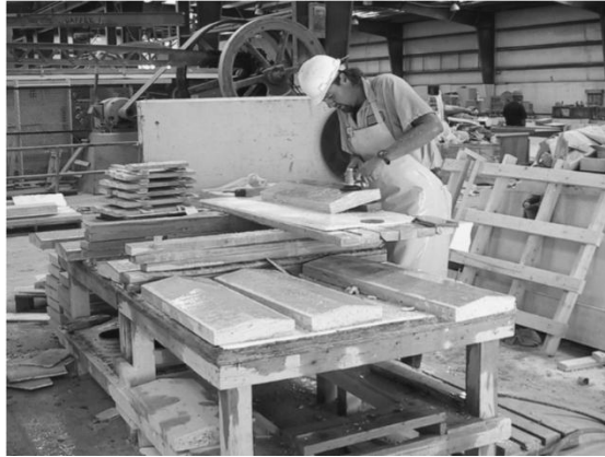
Figure 16.:Limestone capstone being carefully hand-dressed at the finishing plant of New Mexico Travertine, Belen, New Mexico
