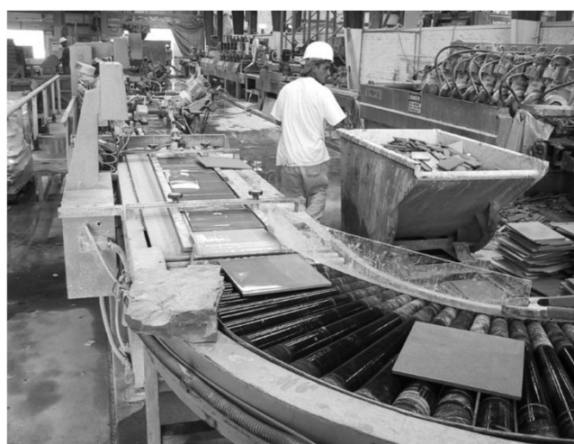
Figure 17. Processing line for square floor tiles at New Mexico Travertine
