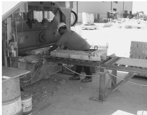
Figure 15: Breaking and palletizing ashlar from dimension stone waste at New Mexico Travertine in Belen, New Mexico
