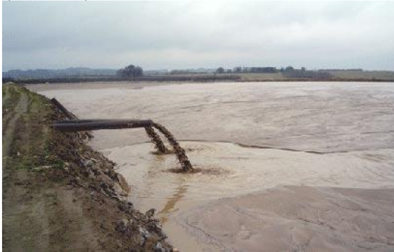
Figure 21 : Single point discharge at Glebe Mines, Derbyshire, England
