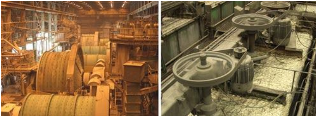
Figure 1: Grinding circuit (left) and froth flotation cells (right) at Highland Valley Copper, BC, Canada
