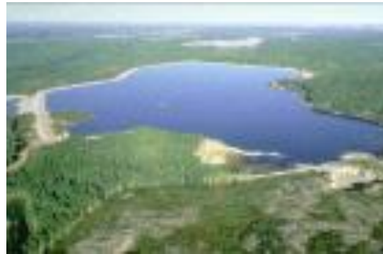
In Figure 24 at the Rio Paracatu Mineracao (RPM) gold mine, Rio Tinto Brazil, the pond has a capacity of 126 million tonnes of tailings and four million tonnes of free water.
