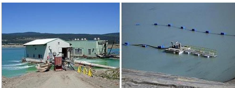
Figure 47: Fixed decant barge (left) and a mobile barge (right)
