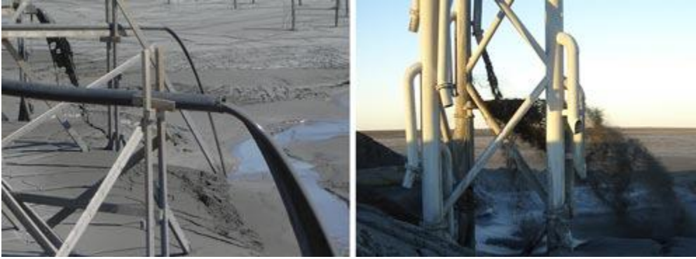
Figure 36: Thickened discharge at Kidd Creek, ON, Canada (left) and at Mt Keith, Western Australia (right)
