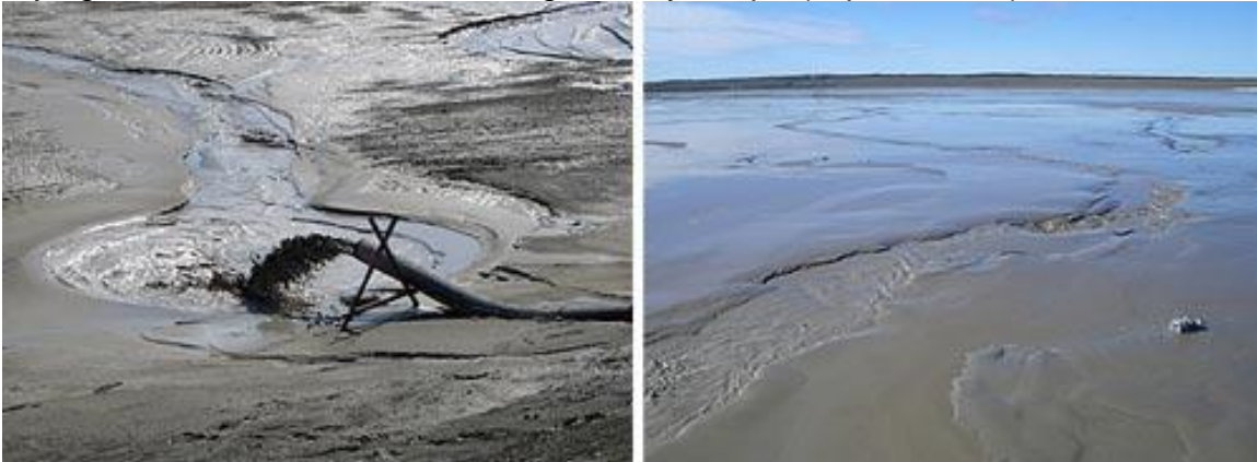
Figure 18: Subaerial tailings discharge (left) and shallow low velocity braided streams on a tailings beach (right)
