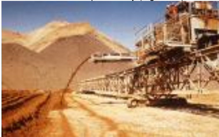
Fig.39: shows conserve water for processing ore so tailings are dewatered and deposited dry in dry climates.
