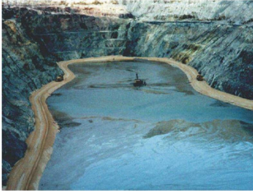
Figure 29. In pit disposal of slurry tailings. (From EU, 2004).
